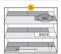
Continue according to this methodology until the last row. Remark: never try to assemble two planks through one single strike!
